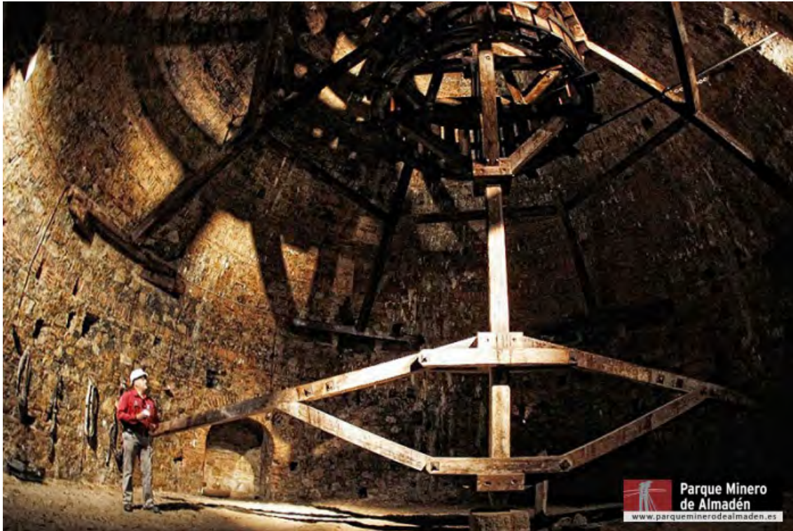
Figure 24. The Baritel (capstan) of the Pozo San Andrés . Source: Parque Minero de Almadén.
