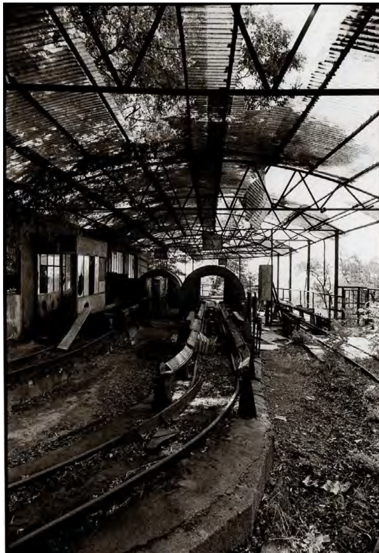
Figure 7. The carousel of wagons at Rostan shaft. Source: Preite, Paesaggi industriali del Novecento , 2006.
