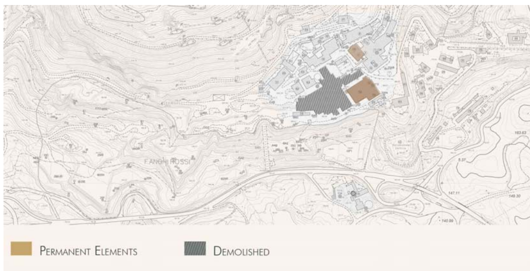
Figure 36 The demolished parts of the Electrolysis plant and the preserved elements.
