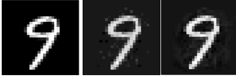
Figure 5.3: Initial digit “9” (left) and its versions modified to be misclassified as “8”. sparse (center) and dense (right) evasion attack samples. Note also how the blurring effect induced by dense attacks is more difficult to spot for humans than the salt-and-pepper noise induced by sparse attacks.
