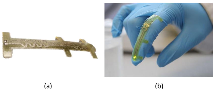
Figure 67. (a) Structure of the 3D inject printed strain sensor and (b) example of bio-application.
