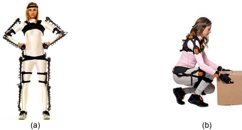
Figure 1.2 Non-optical motion capture systems: (a) the Gypsy 7 mechanical suite (CA, USA, http://metamotion.com ) and (b) the Xsens MVN inertial motion capture suite (Xsens, Netherlands, http://www.xsens.com ).
