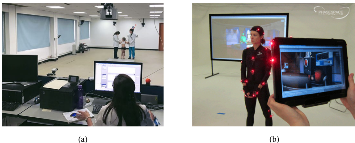
Figure 1.1 Motion capture systems: (a) a passive marker-based motion capture system by BTS Bioengineering (Italy, http://www.btsbioengineering.com ); (b) an active marker-based optoelectronic system by PhaseSpace Inc. (CA, USA, http://www.phasespace.com ).
