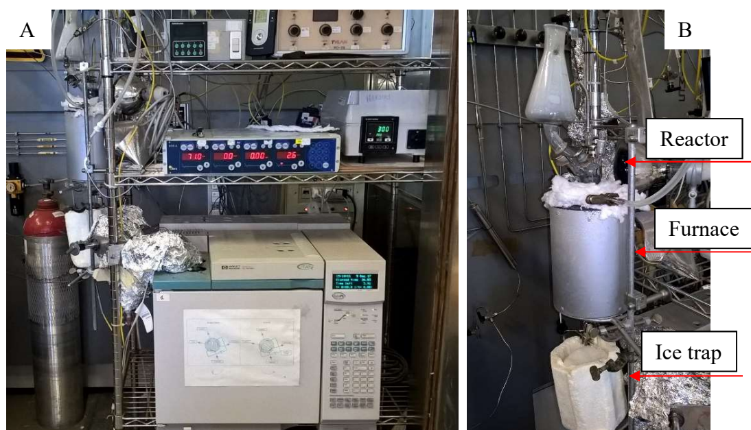
Fig. 2.2. CO 2 to methane plant and gas analysis system (A); Reactor and furnace (B).
