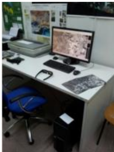
Figure 57 Digital Photogrammetric Workstation or Softcopy Workstation, 3D vision: NVIDIA 3D Vision® 2 with a USB IR Emitter and a 3D LCD monitor ASUS.
