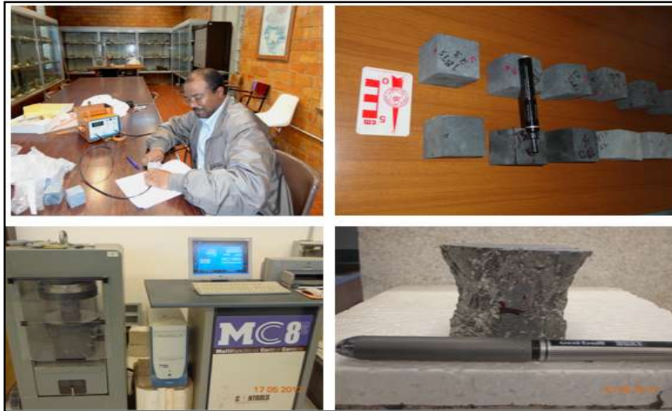
Figure 12-4 Determination of Uniaxial Compressive Strength and ultrasonic Velocity in the laboratory
