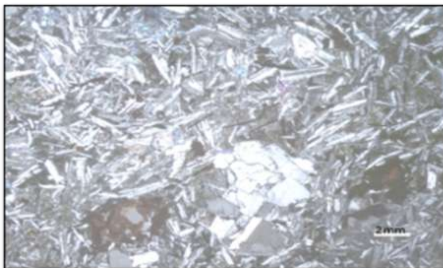
Figure 11-9 Microscopic photo under crossed nicol, x10, showing the andesitic rocks with abundant laths of plagioclase and rare olivine phenocrysts which are oxidized
