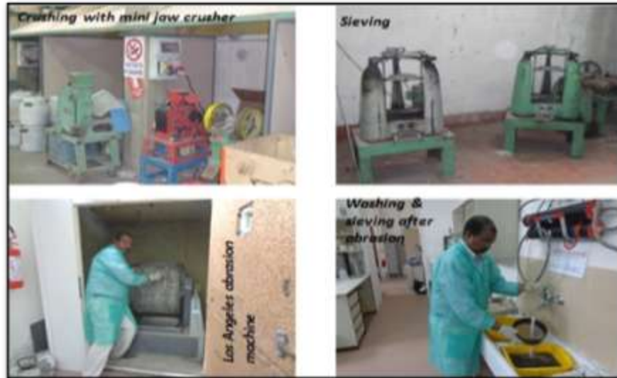
Figure 13-6 Photo showing the steps followed in Los Angeles Abrasion Value testing
