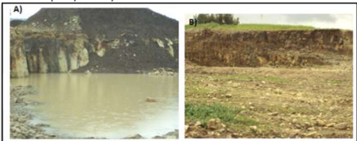
Figure 7-5 Dimension stone quarry in the studied area, A) Ponds created due to poor drainage system and displacement of the fertile black cotton soil, B) Selected material quarry affecting farm land
