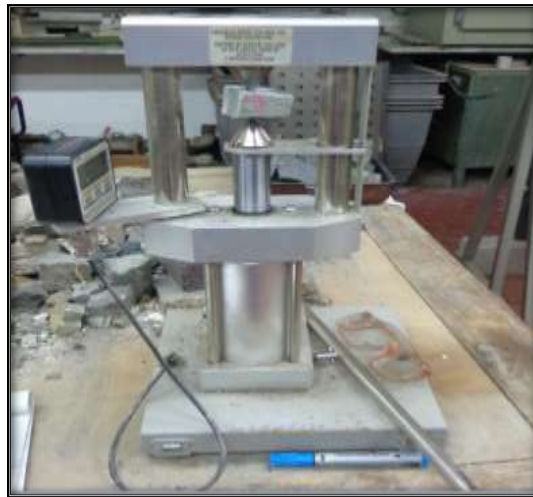
Figure 5-13 The Point Load Test machine used in this study
