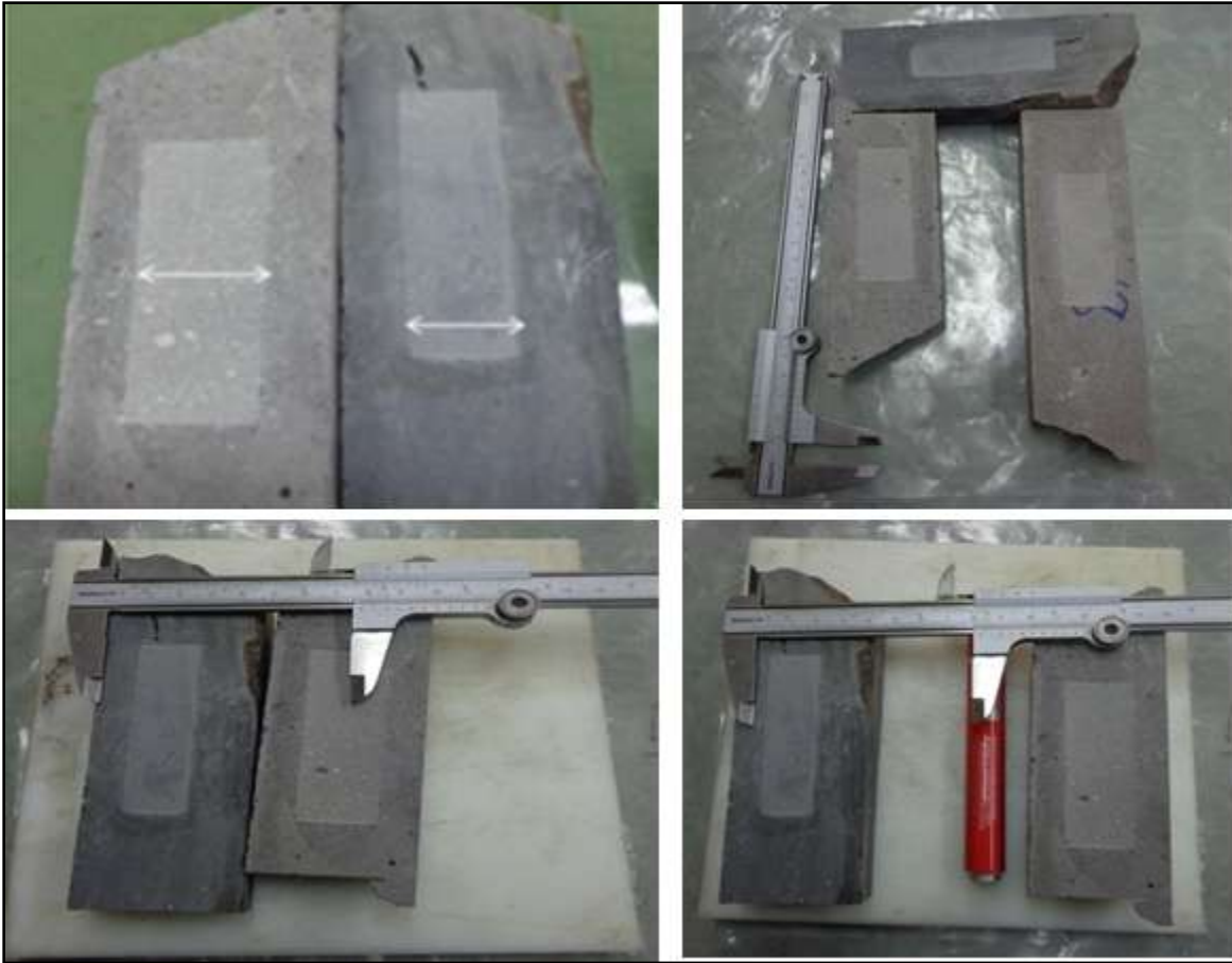
Figure 12-12 The different lithotype abrasion test result patterns (grooves made by the abrasion Capon wheel)
