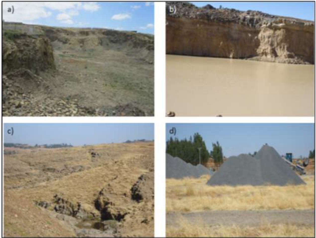
Figure 7-6 Aggregate quarry impacts, a) Abandoned quarry, b) Abandoned selected material quarry creating ponds, reported by the local people, 2 children were died by drowning in the pond, c) Adjacent streams polluted with sediments and suspended materials, d) Stockpiles on grasslands creating land use problem.
