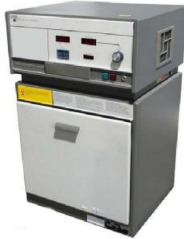
Figure 4-8: X-radiography inspection system.
