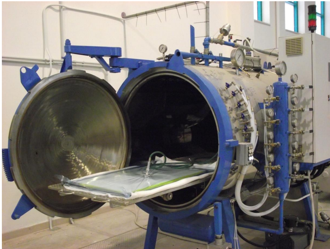
Figure 4-4: Vacuum bag sequence and tool plate placed in an autoclave.
