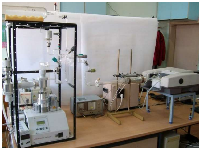
Figure 2.8. The whole apparatus for adsorption FTIR experiments.
