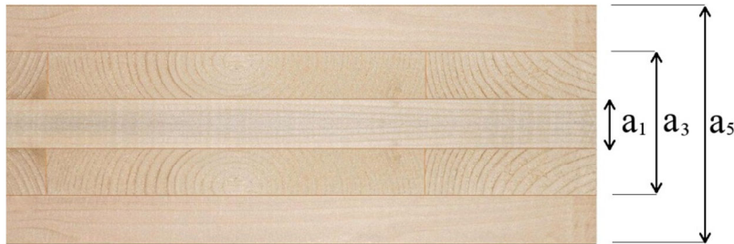
Figure 3-26 Definition of various thicknesses in a generic 5-layer CLT panel (after Follesa et al., 2013).
