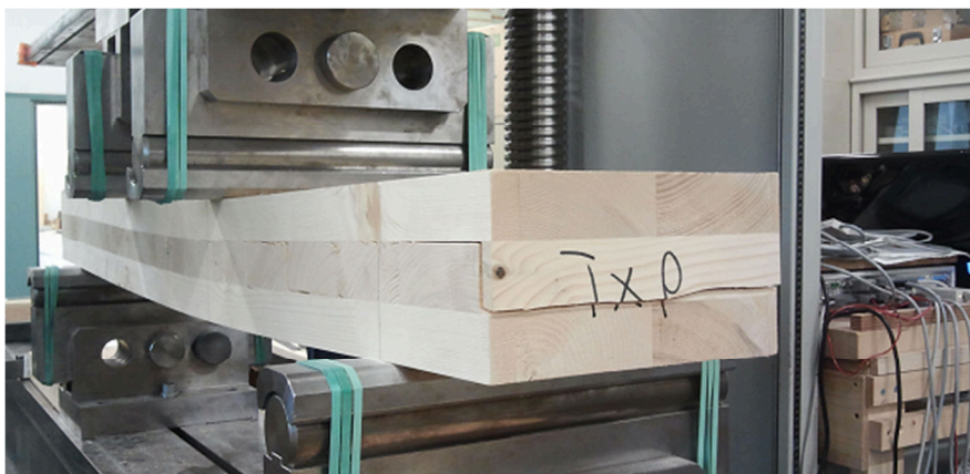
Figure 3-5 Out-of-plane bending test of the CLT panel. Test set-up and execution.
