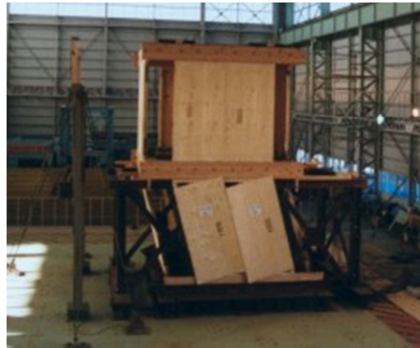
Figure 3-88 Slip behaviour of wood-based sheathing with respect to the timber frame and collapse reached in a light-frame building subjected to a shaking table test.
