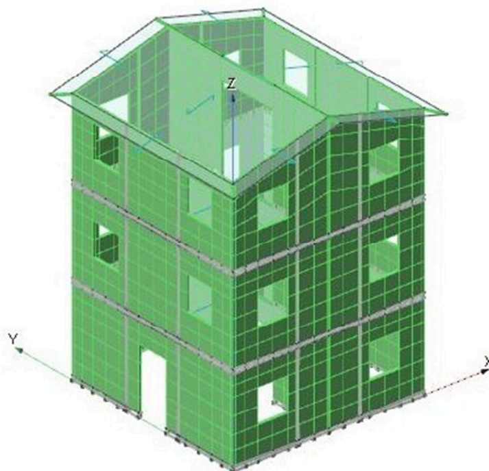
Figure 3-39 Undeformed shape of the FE model (after Follesa et al., 2013).
