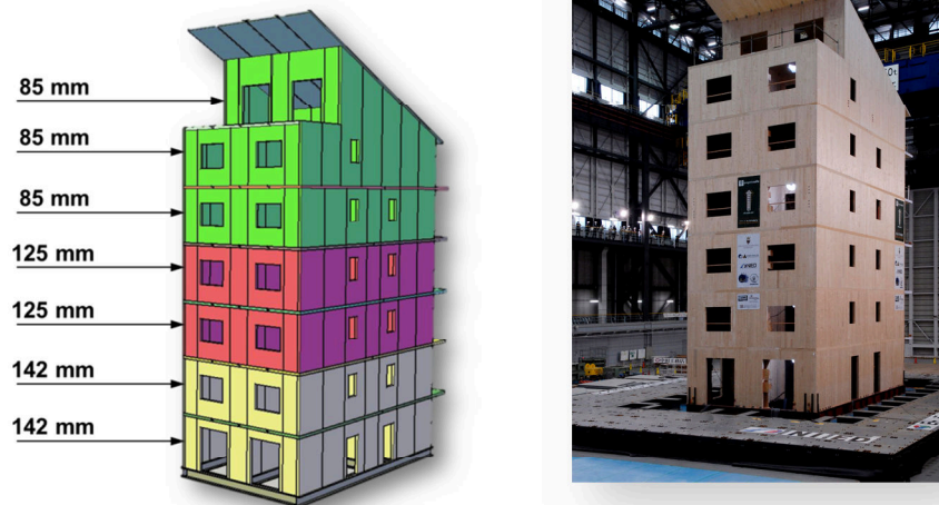
Figure 1-6: Shaking table tests of a seven storey CLT building conducted in 2007 in Miki (Kobe), Japan within the Sofie Project. Specimen layout with wall thickness at each storey (floors were all made with 142 mm CLT panels) and picture of the specimen over the shaking table (right).
