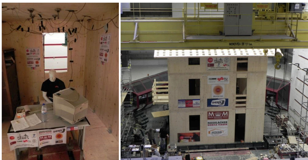
Figure 1-11: Shaking table tests of a three storey CLT conducted in 2011 in Lisbon, Portugal within the SERIES Project. Accelerometers placed inside a monitored room and picture of the specimen over the shaking table (after Campos Costa et al., 2013d).
