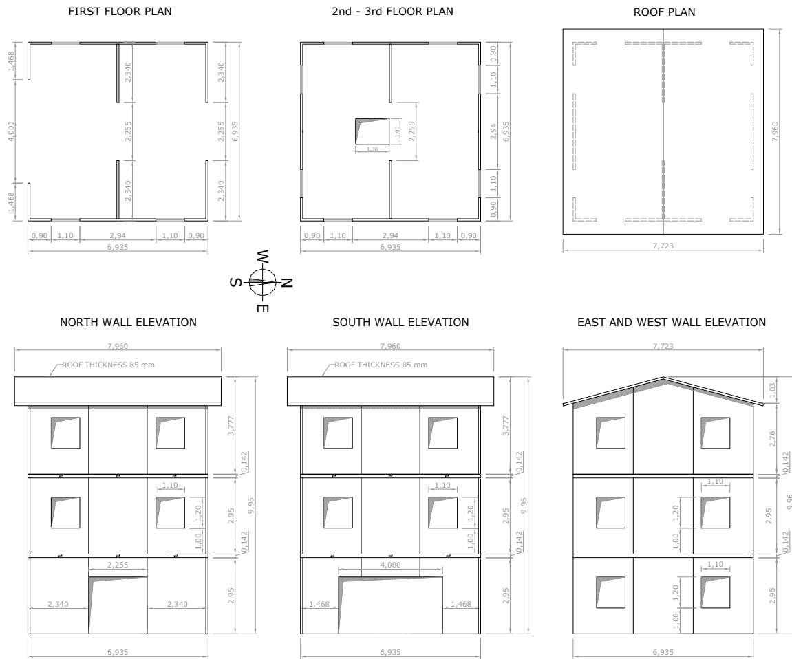
Figure 3-33 Plans and elevations of the case study building (dimensions in m) (after Follesa et al., 2013).
