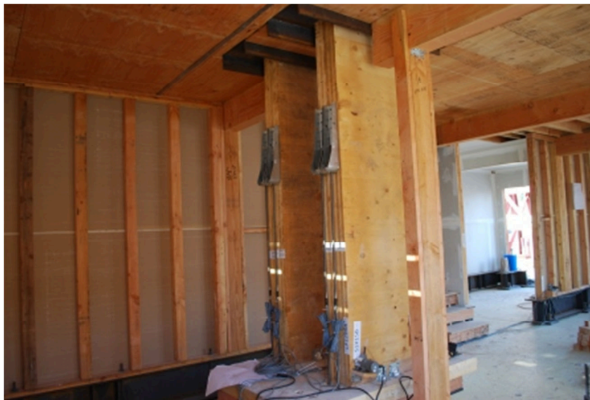
Figure 1-12: Specimen retrofitted with CLT rocking walls according to FEMA P807 guidelines before the shaking table tests.
