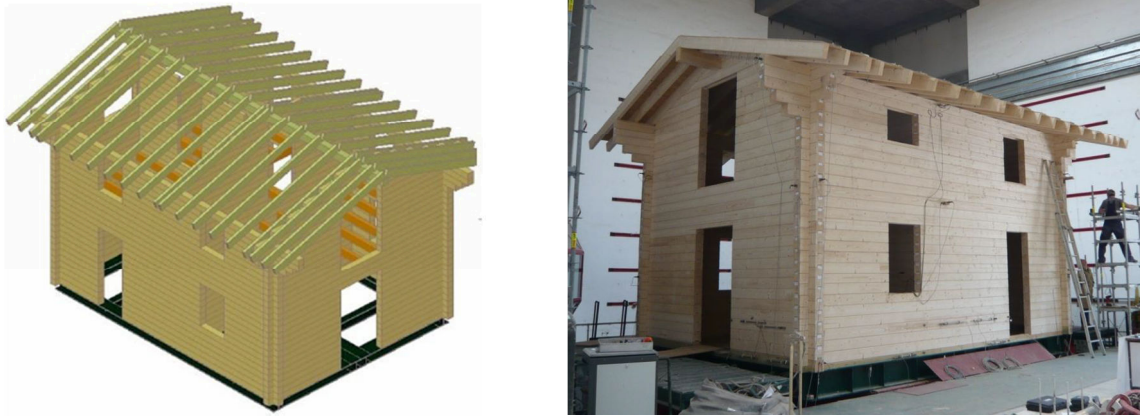
Figure 1-8: Shaking table tests of a two storey Log House building conducted in 2011 in Lisbon, Portugal within the SERIES Project. 3D model of the specimen and picture of the specimen over the shaking table (after Campos Costa et al., 2013a).
