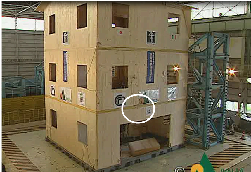
Figure 3-16 Uplift of the middle panel in 2 nd story wall (marked with the white circle) and corresponding slip of the vertical step joint observed during the 100% JMA Kobe (0.82g) test on a three story CLT building performed within the SOFIE Project at the NIED shaking table facility in Tsukuba, Japan, July 2006 ( www.progettosofie.it ).
