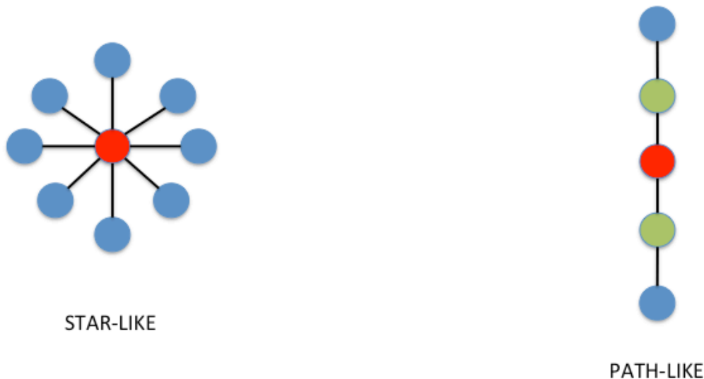
Figure 7 Schematic representation of minimum spanning tree (MST). Examples of star-like and path-like topologies. Blue nodes represent leaves. In the star-like topology the red node is the node with higher betweenness centrality (it is equal to 1) and higher degree (it is equal to 8) and lowest eccentricity (it is equal to 1). All the other nodes in the star-like topology have degree=1, eccentricity=2 and betweenness centrality=0. In the path-like topology red node characteristic are degree=2, betweenness centrality=0.5 and eccentricity=2. Tree characteristic in star-like topology are diameter=2, leaf number=8 and tree hierarchy=0.5. In path-like topology, red node characteristics are: degree = 2, BC = 0.5, and eccentricity = 2. The tree characteristics are leaf number = 2, tree hierarchy = 0.5, and diameter = 4. Adapted from [137].
