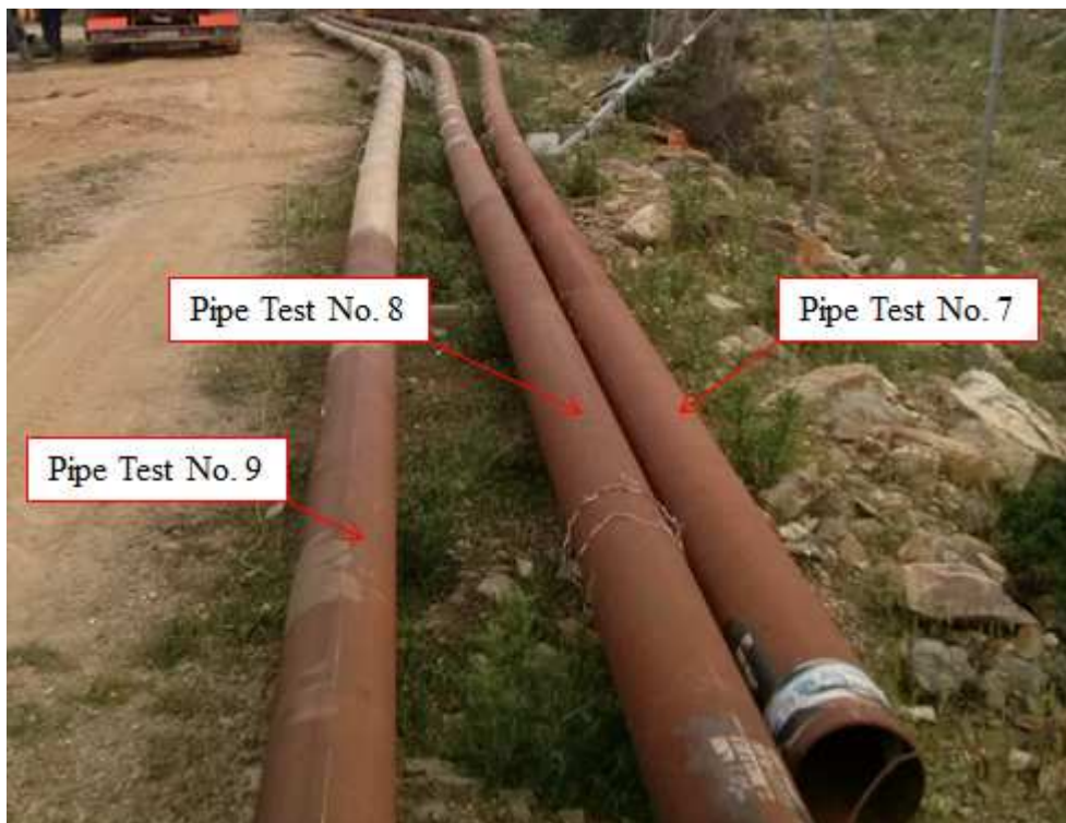
Fig. 146. Pipe final deformation after the Test No. 9, Test No. 8 and Test No. 7.
