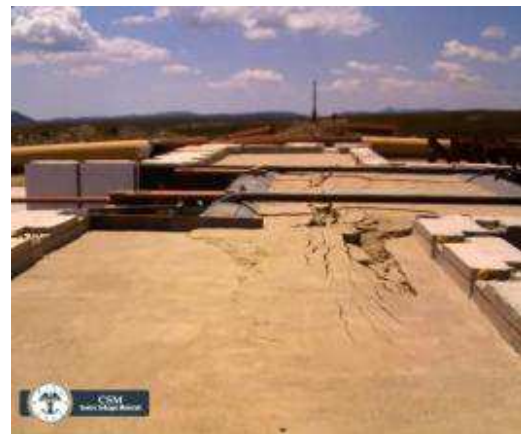
b) Upper soil surface at 1800 mm of caisson displacement.
