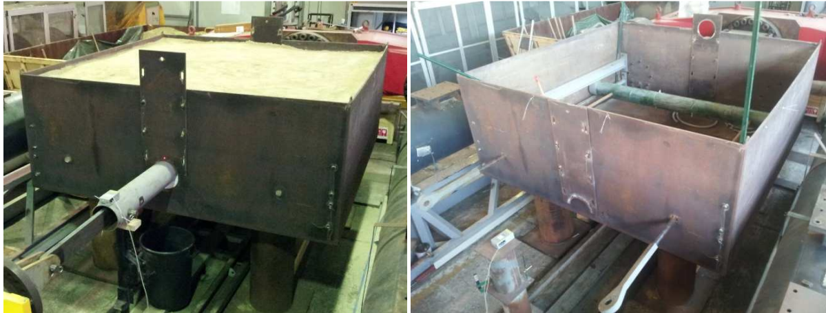
b). Lateral pullout configuration (with removed sand).
