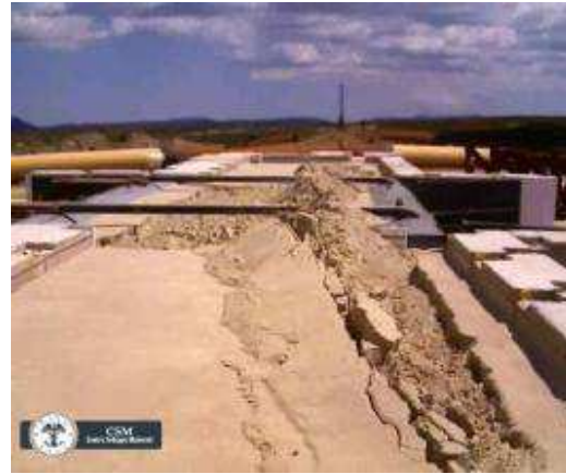
d) Upper soil surface at 3650 mm of caisson displacement.
