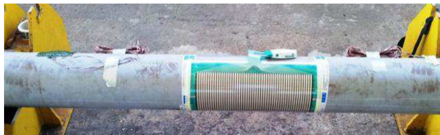
Fig. 21. Pressure sensor wrapped on pipe.
