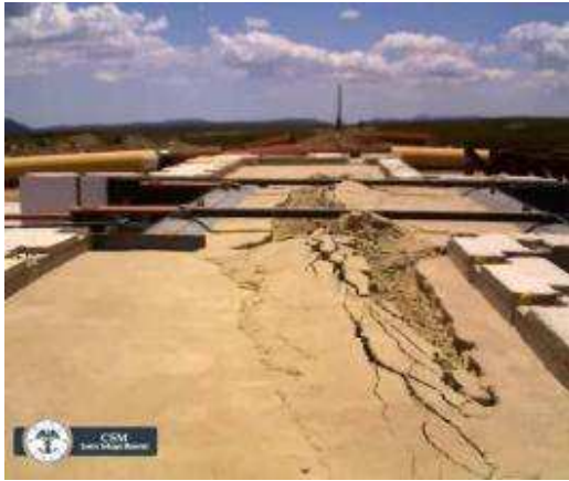
c) Upper soil surface at 2800 mm of caisson displacement.
