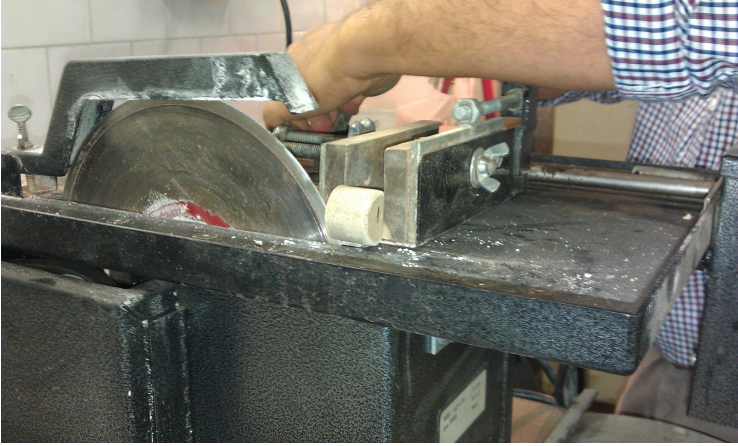
Figure 4.9. Saw cutting of the samples.
