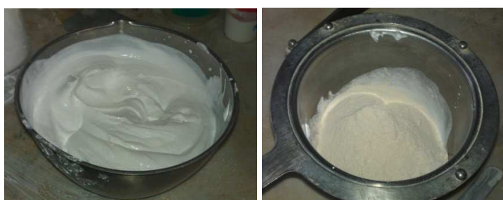
Figure 4.17. Preparation of lime putty (left) and collection of CFP (right).
