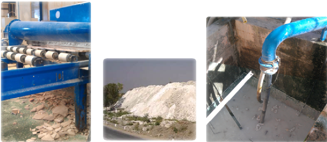
Figure 3.1. From the left: rejected stone fragments and trimmings (CC); dust and fine powder (CSG); slurry from the filter press (CFP).
