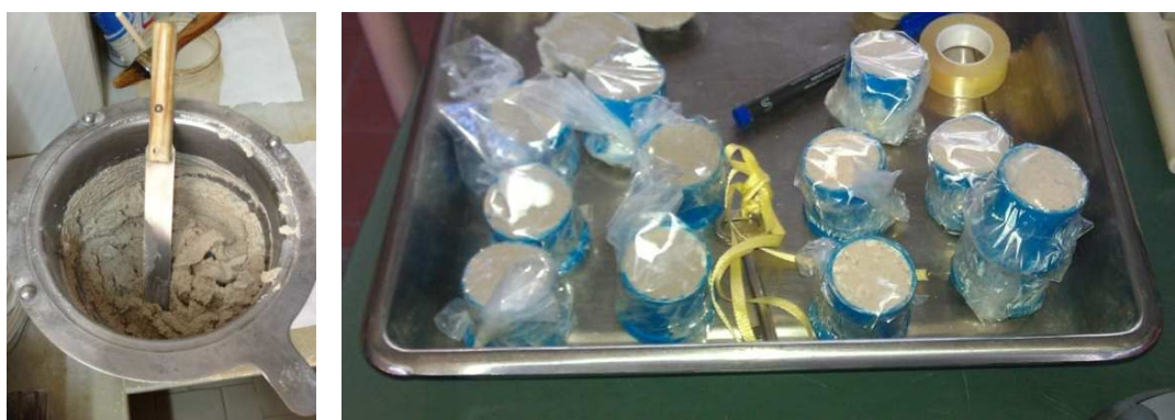
Figure 4.6. Preparation of mortars (left) and plastic moulds (right).
