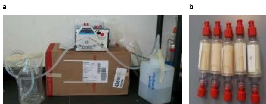
Figure 1.2. On-field processing of seawater samples for DNA extraction. a) Seawater filtration apparatus. b) Sterivex GP cartridge.
