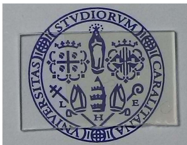
Figure S8. Picture of a GLYMO-based silica thin film doped with 2 obtained by dip coating.
