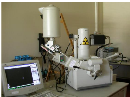
Figure 9: Scanning Electron Microscopy (SEM) equipped with Energy Dispersive X-Ray (EDX) detector (Zeiss, Germany).
