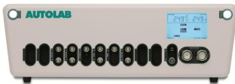
Figure 8: Autolab 302N potentiostat-galvanostat controlled by NOVA software (Metrohm, Switzerland).
