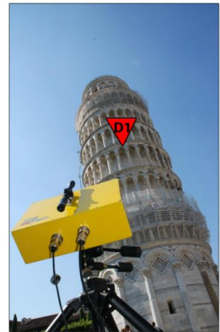
Figure 4.6: Frequency composition of the signal reflected from the points at middle height of the tower for the measure positions B, C and D and their identification on pictures with the same viewpoints of the operating IBIS-S. All the measurements are collected with only wind energization.
