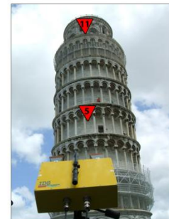
Figure 4.3: Power profile and selection of measuring points: it is important to distinguish between peaks power on metal scaffolding and those really belonging to the structure
