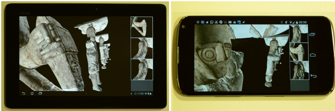
Figure 8.1: Remote inspection. Remote virtual exploration of a scene composed by several high resolution statues on a Asus TF201 tablet (left image), and on a LG Nexus 4 smartphone (right image). During interaction, models are adaptively downloaded from the network, and knowledge of the currently rendered scene is exploited to automatically center a rotation pivot for the camera controller and to propose context-dependent precomputed viewpoints.
