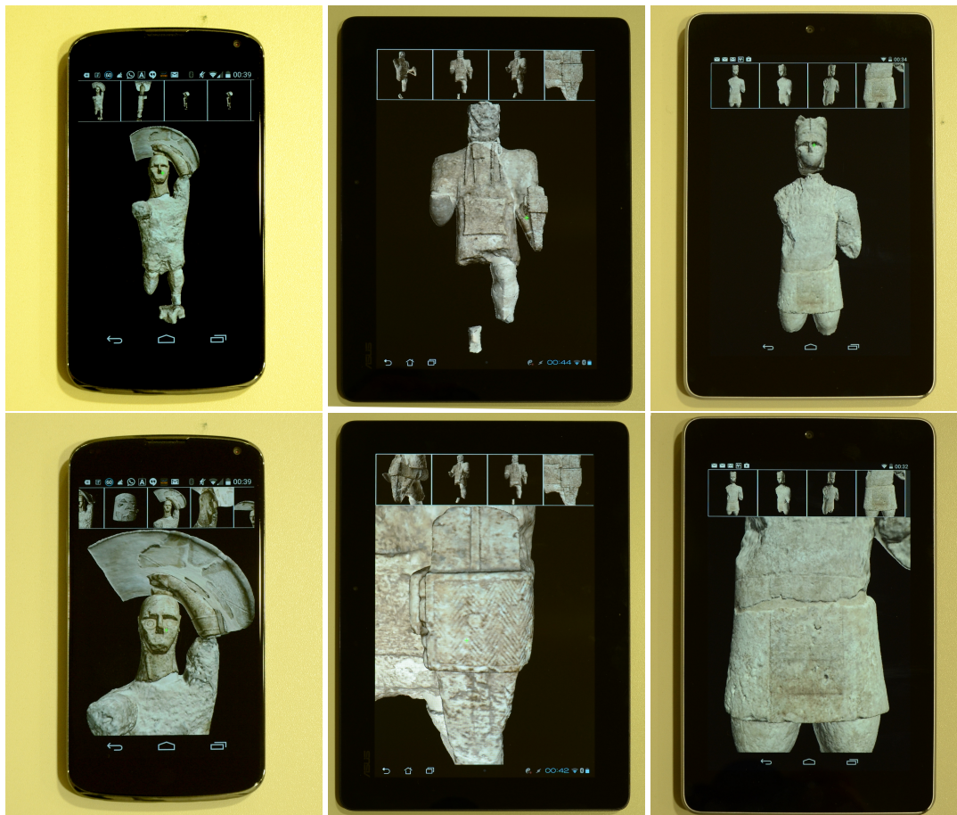
Figure 8.7: Various levels of detail of a statue. Images correspond to Nexus 4, Asus TF201 and Nexus 7, respectively. Top: View of the whole statue. Bottom: A close-up of the statue showing small-scale details.
