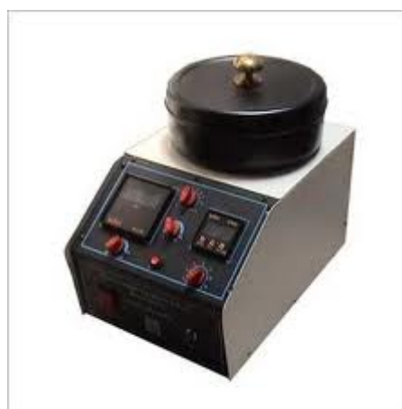
Figure A.6: thin glass support (left) and the spin coater (right) used in this work.
