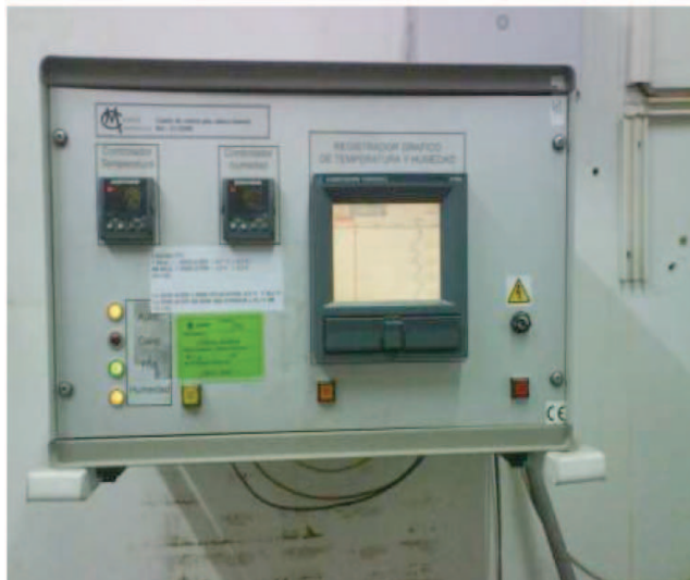
Figure 5.8: Console of regulation of environmental conditions in the moist chamber. (Martin, J. 2010).
