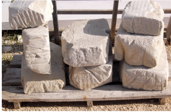
Figure 8.1: Experimental cellular blocks after demolding.
