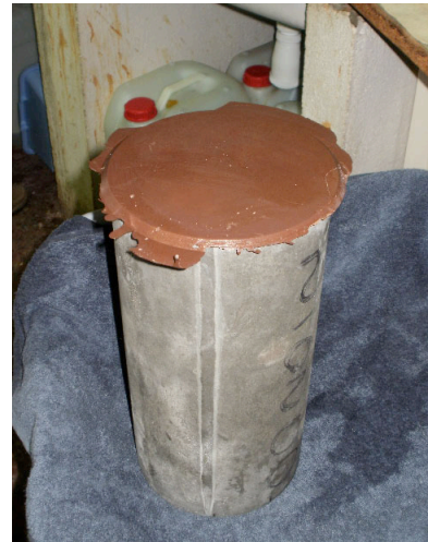
Figure 5.9: Specimen into a pool of molten sulfur mixture. Figure 5.10: Capped specimen.
