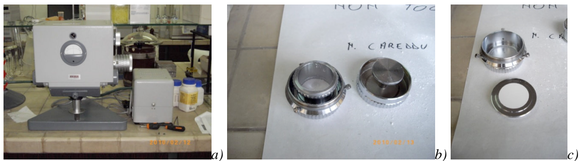
Figure 4.5: a) Photoelectric Reflectance Photometer ELREPHO; b) Sample dish mould; c) Powder sample dish.
