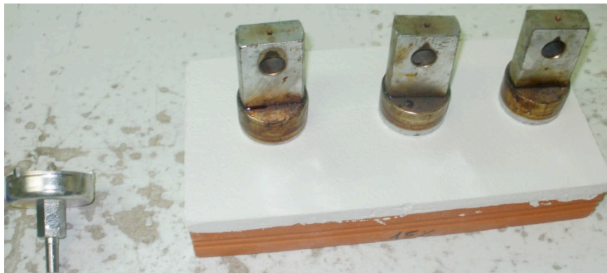
Figure 7.7: Pull-heads for the adhesive test.
