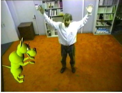
Figure 1.1: The virtual world in Alive is composed of image in real-time of user with computer graphics [144]. The figure shows a virtual dog which mimics user's gesture.
