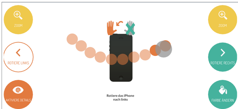
Figure 2.8: An example of gesture guiding in ShapelineGuide [3]: the hand-icons, located above the smartphone, indicate which hand the user has to use; the gesture's path is described using a sequence of orange circle subdivided in more segments.
