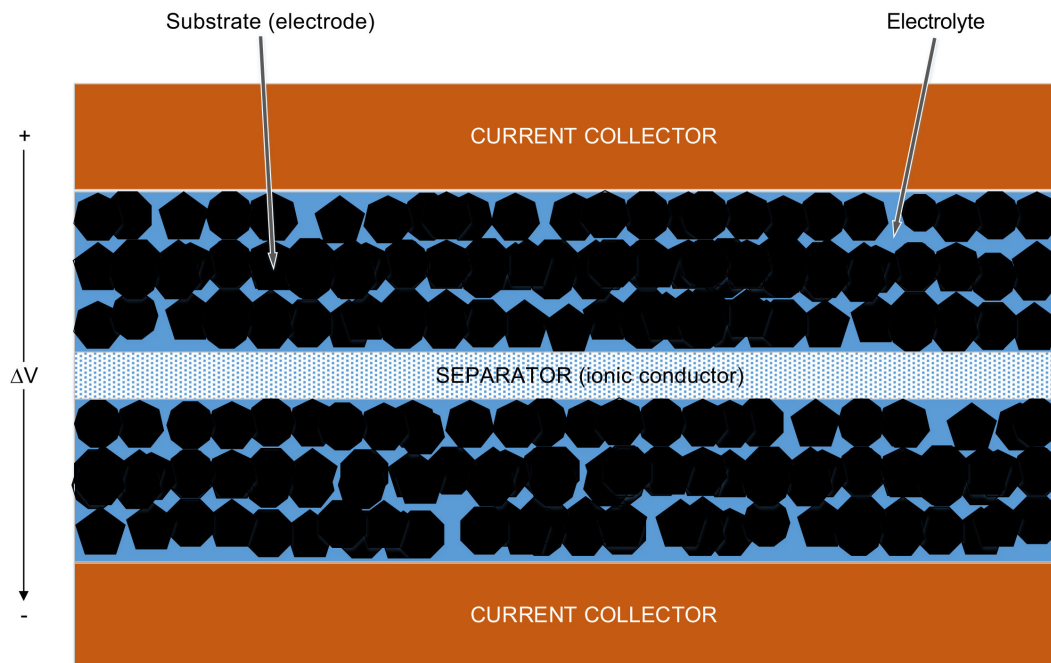
Figure 1.6: Schematic diagram of a super-capacitor. Original schematic is from [3].
