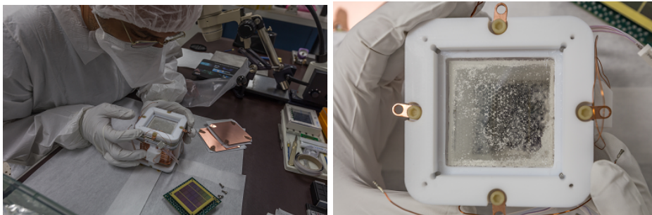
Fig. 4.8: Degradation of the TPB deposition on acrylic substrate. It can be seen the strong TPB degradation on top window, even with little TPB flakes on the grid.
