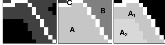
Fig. 2.4. Segmentation and edge areas labeling. From left: original feature-map, result of labeling, region weighting for the considered area
