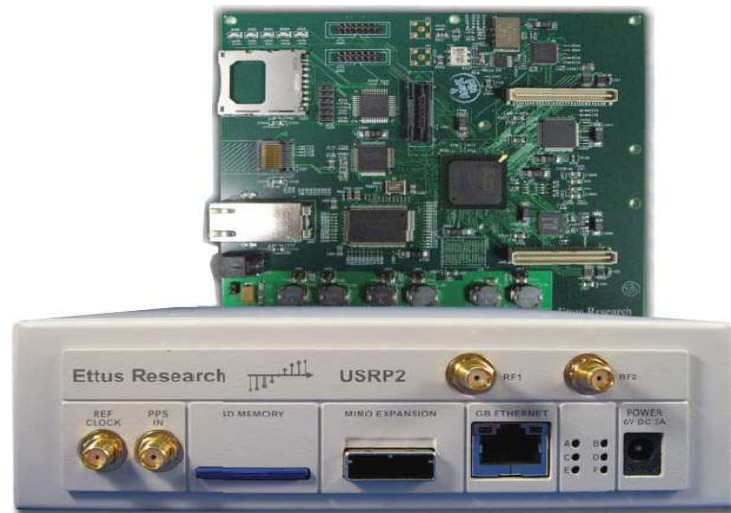
Figure 7 Universal Software Radio Peripheral 2 (USRP2) SDR.
