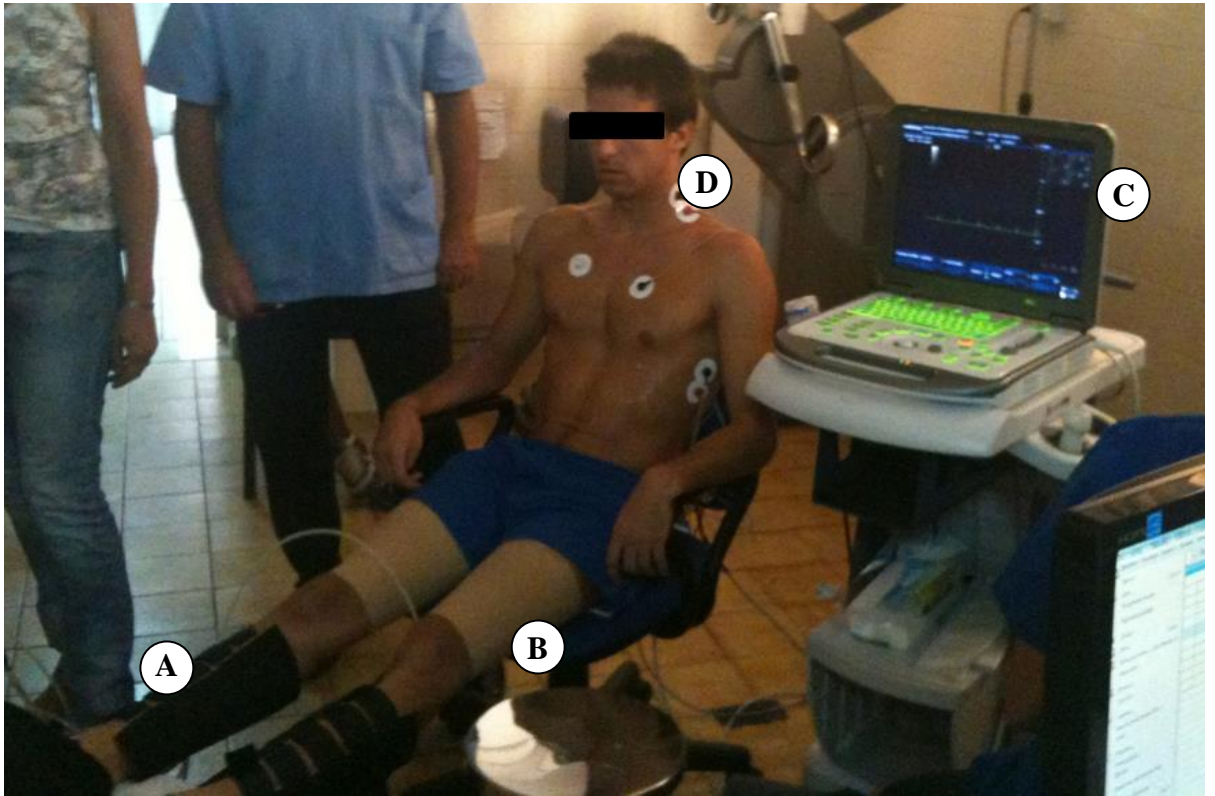
Fig. 15. One of the subject in the study wearing the automatic device (A) and elastic sleeve (B). Echocardiographer (C) and impedance cardiometer (D) placed on the neck and chest can be seen during data collection.
