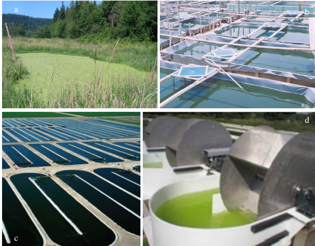
Figure 3. Example of open cultivation systems: a) natural unstirred pond (Wikipedia, 2011), b) small pond for Spirulina culture, Asia (Wikipedia, 2011), c) Open raceway-type culture ponds of Earthrise in California, US (Spirulina.org.uk), d) Paddle wheel of a raceway pond (Department of Chemical Engineering, Tehran Polytechnic, Iran)
