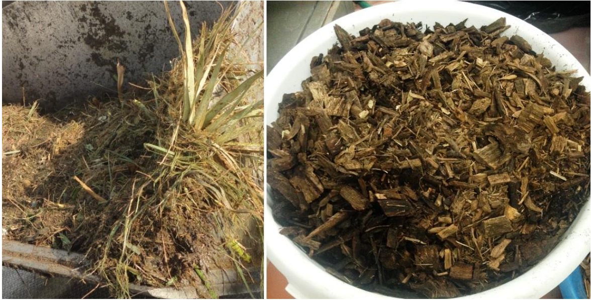
Fig. 4.5. The bulking material employed in the pilot-scale (grass and tree prunings, left) and laboratory-scale (wood chips, right) experiments.
