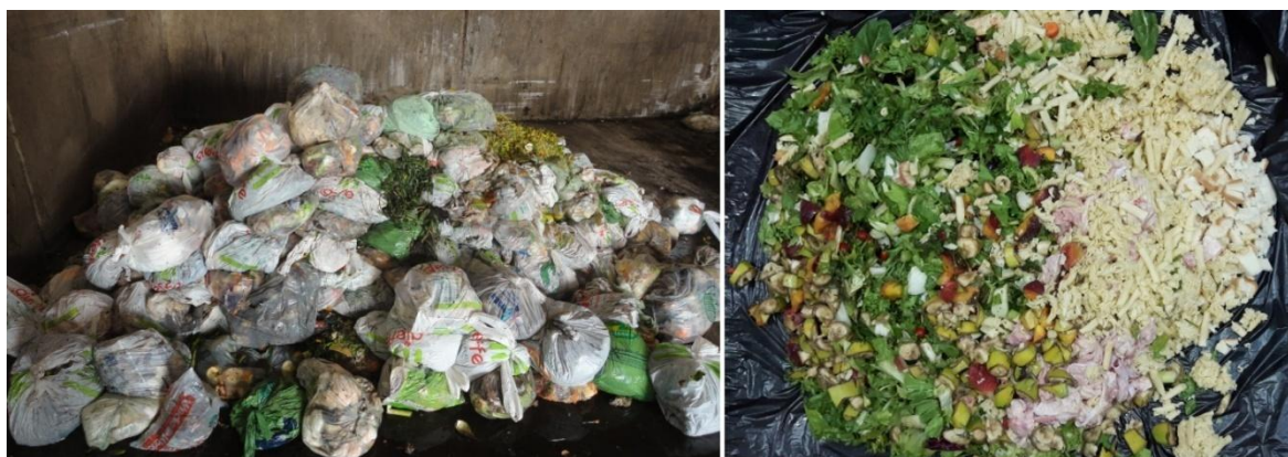
Fig. 4.4. The organic fraction of the municipal solid waste (OFMSW) employed in the pilot-scale (left) and laboratory-scale (right) experiments.
