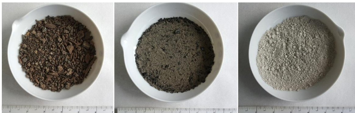
Fig. 3.2. The biomass combustion residues: BTA (left), BOA (center) and FA (right).
