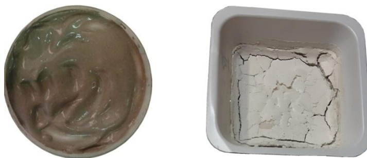
Fig. 5.5. Fly ash before (left) and after (right) the accelerated carbonation treatment.
