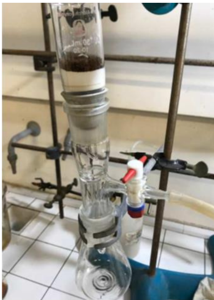
Figure 11 Filtration of crude mixture on a short pad of silica
