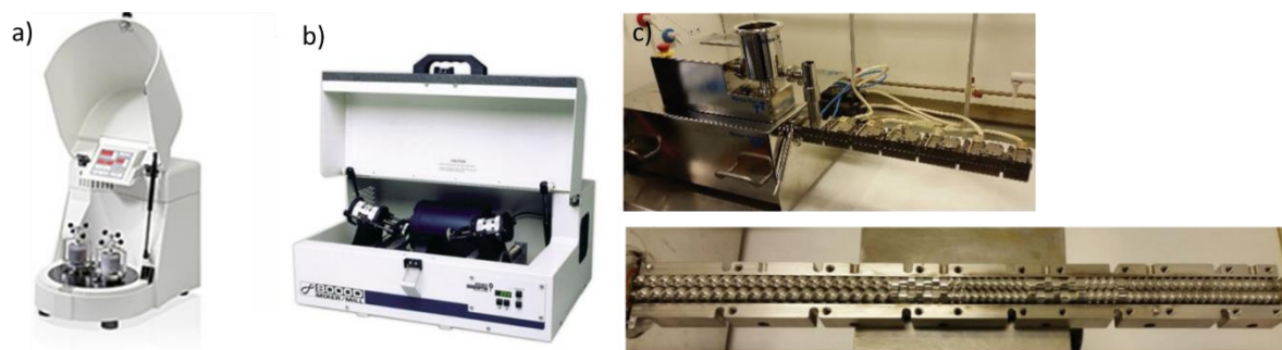
Figure 1 a) Planetary Micro Mill PULVERISETTE7- FRITSCH (b) 8000M Mixer/Mill® - SPEX c) Twin screw extruder and intermeshing co-rotating screws Reproduced from Ref. 32 with permission from The Royal Society of Chemistry
