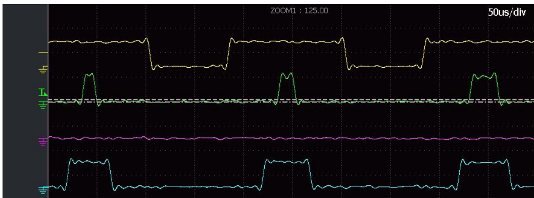
Figure 106: Modulation control signals of prism 1 tetrahedron 1.
