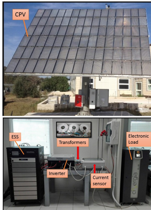
Figure 28: CPV power plant (top) and MG test bench (bottom).
