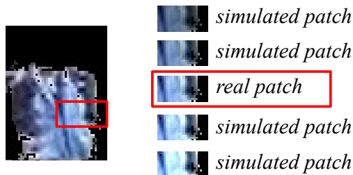
Figure 4.3: Examples of four artificial patches simulating changing illumination (right), corresponding to the patch highlighted on the left.
