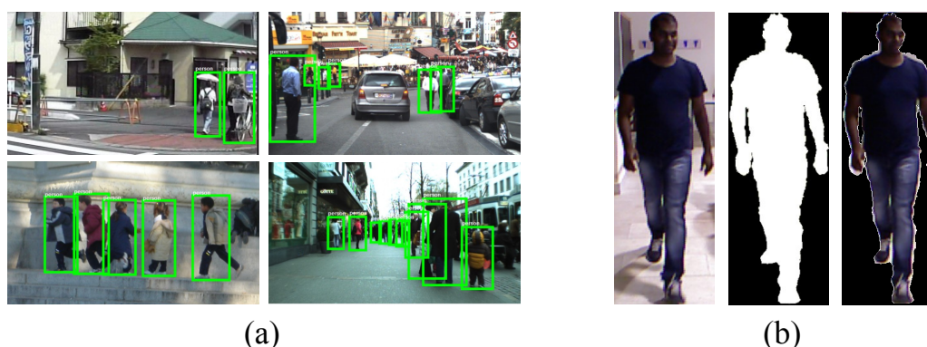
Figure 2.1: (a) Example outputs of a pedestrian detection algorithm in three frames taken from real-world video-surveillance footages; Detected blobs are in green. (b) Example of division of a blob into person and non-person pixels.
