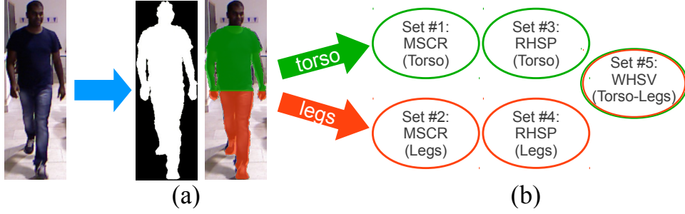
Figure 3.2: The popular SDALF descriptor [45] as an instantiation of the proposed appearance model. SDALF subdivides body into torso (disregarding the head) and legs parts (a); from each part, RHSP and MSCR local features are extracted, and the weighted HSV histograms of each part are concatenated, leading to five sets of components (b).
