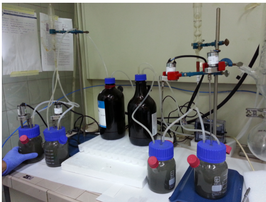
Figure 3.13 Example of batch tests performed in the current study. Each reactor was covered with aluminium foil in order to avoid photo-oxidation effects.
