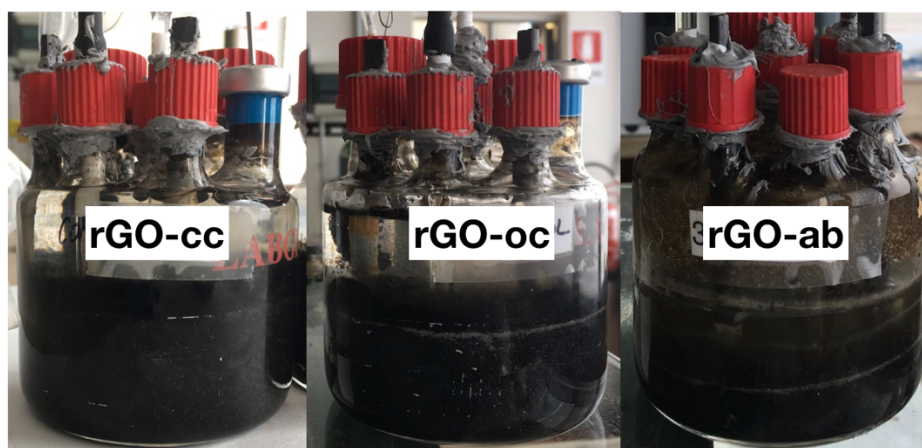
Figure 4.28 Digital picture of the SBESs adopted in this study: rGO-cc was operated in closed circuit, while rGO-oc and rGO-ab were operated in open circuit (glutaraldehyde was added to rGO-ab in order to kill the biomass within the reactor).
