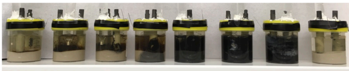
Figure 4.16 Digital picture of a representative test of electro-reduction (after 60 hours); from the left to the right: test-tubes amended with GO concentrations from 10 \text{ mg}_{GO} \text{ kg}_{dw}^{-1} to 2,000 \text{ mg}_{GO} \text{ kg}_{dw}^{-1} , and control without GO amendment (last tube on the right). The picture shows that, in this specific configuration, GO concentrations below 500 \text{ mg}_{GO} \text{ kg}_{dw}^{-1} were not enough to create a visible reduction in the whole volume.
