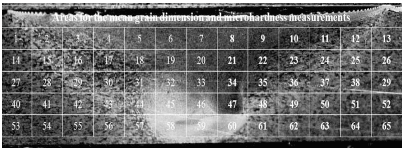
Fig. 10 - Grid of mean grain and micro-hardness measurements.
