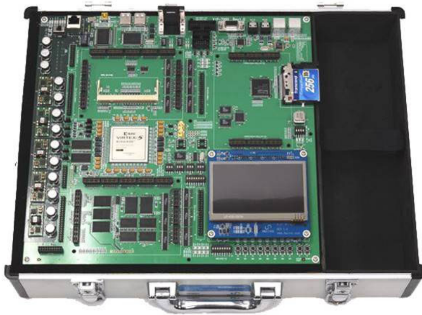
Figure 3.5: Virtex5-based prototyping board
