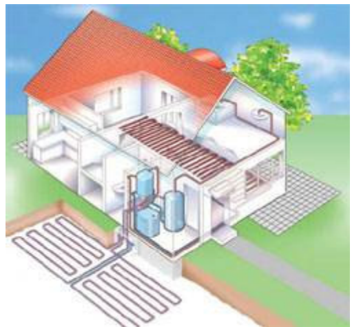
Figure 6: Geothermal horizontal loops (source: ACCLIMATIZE 2010)
