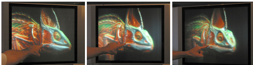
Figure 5.4: Volume ray-casting results with the chameleon dataset. Images of the light-field display taken with a hand held video camera moving in the display workspace. Note the parallax effects and the view-dependent illumination effects.
