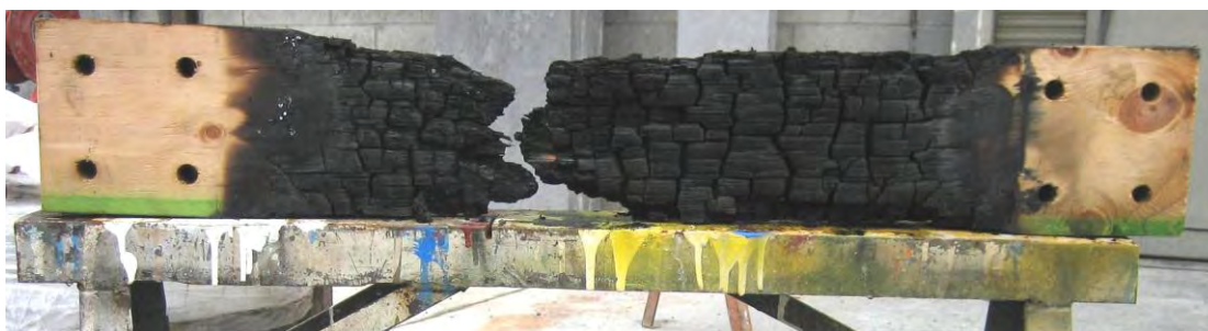
Fig. 3.6 - Typical brittle failure of specimens loaded in tension.
