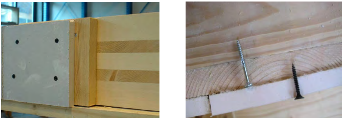
Fig. 5.16 - Protection of specimen lateral edges with gypsum plasterboard and wood.
