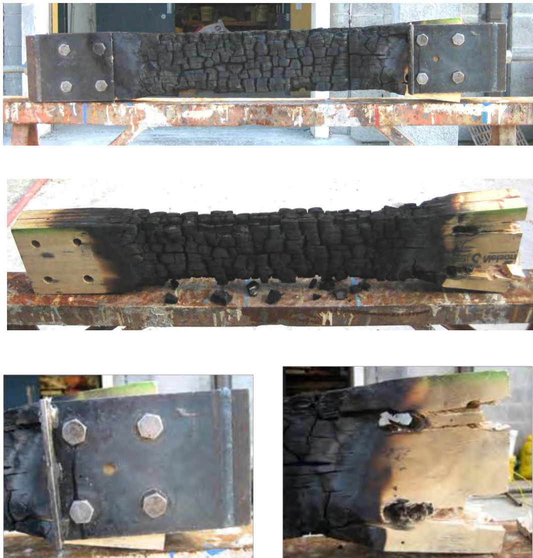
Fig. 3.7 - Failure close to the connection with the steel support.
