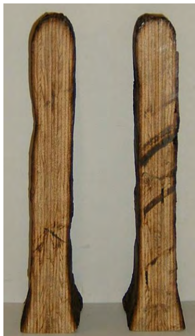
Fig. 2.11 - Two slices of the residual section of the specimen 3 tested in the pilot furnace [Lane 2005].
