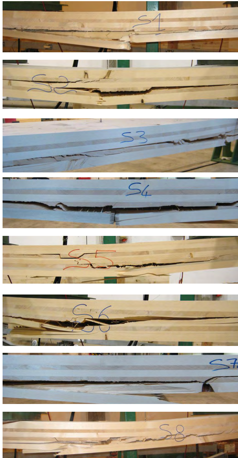
Fig. 5.9 - Failure in bending of XLAM panels of series 'S' at ambient conditions.
