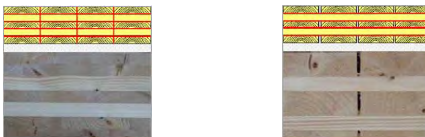
Fig. 4.2 - XLAM cross-sections with glued board edges (left) and no glued board edges (right) [Promo_legno].
