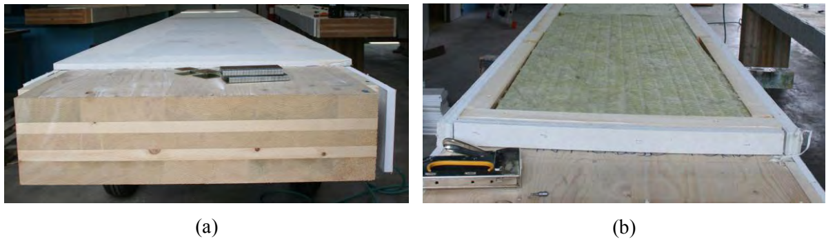
Fig. 5.15 - (a) Specimen S3-IV protected with gypsum fibreboard. (b) Specimen S3-III protected with gypsum fibreboard and rock wool.
