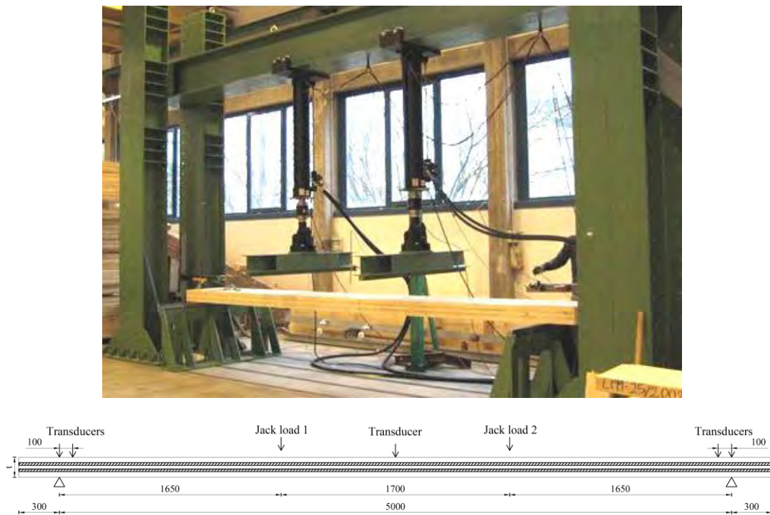
Fig. 5.3 - Photo of a specimen before the bending test at ambient condition (top) and setup of the test with dimensions in mm (bottom).
