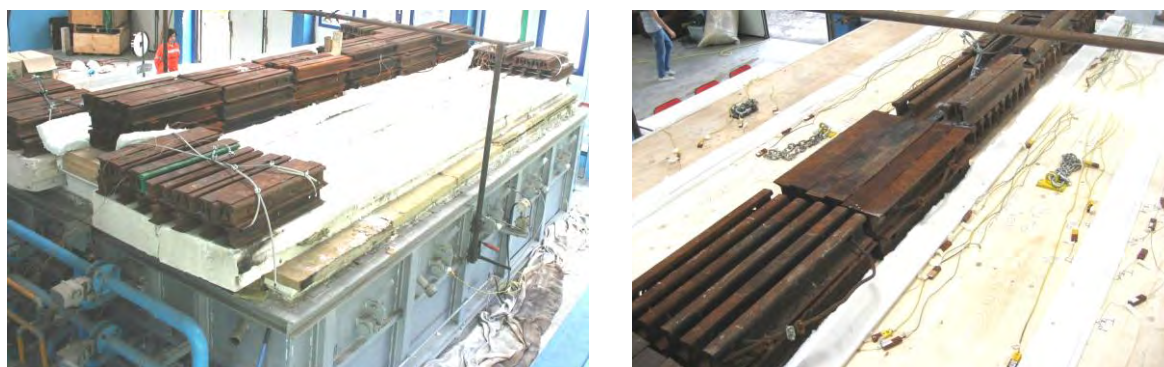
Fig. 5.17 - Photos of fire tests No. 1 (left) and No. 3 (right). The loaded specimens are in the centre of the furnace, and the unloaded precast concrete/XLAM panels are besides (left/right photo).
