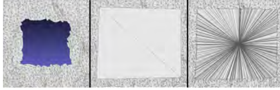
Figure A.8: Test case. A hole in a dense mesh (left) is covered with with a quad (center) and the algorithm produces a conformal mesh.
