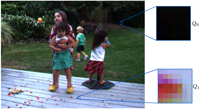
Figure 1.8: Two patches (or region) Q_0 and Q_1 , selected on an input image, both having 7 \times 7 pixels size. The patch Q_1 contain enough information to estimate the motion of its pixels, while the patch Q_0 as poor texture, and therefore will not produce reliable results.
