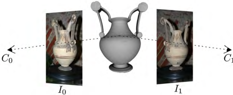
Figure 2.1: The same object (in this case, a vase) captured from two different viewpoints, and a digital representation encoding only the geometry on the object. Our goal is to find the correct alignment of the cameras in order to project the color and texture information from the image onto the surface. See also Figure 1.2 for a similar case.
