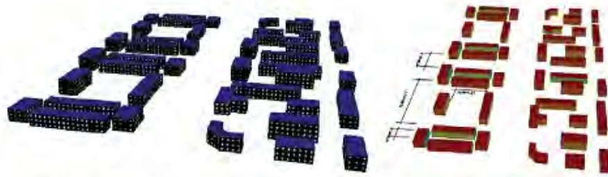
Layout of case study site (left), with facades falsecoloured according to incident annual solar irradiation (right).
