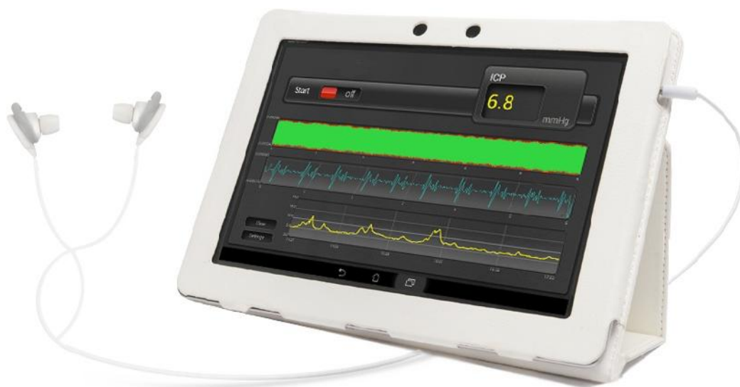
Fig. 4.9: NI-ICP monitoring algorithm and visual interface on a dedicated tablet
