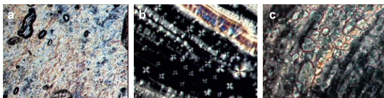
Figure 4.3: Optical microscopy: (a) Typical sample, containing 5 wt % of W, in the LC H_2 region of the LCT/GTO 90/10 mass ratio line. (b) Sample containing 25 wt % of W in the emulsion region for the LCT/GTO 90/10 mass ratio. (c) Sample containing 20 wt % of W in the emulsion region for the LCT/GTO 85/15 mass ratio.
