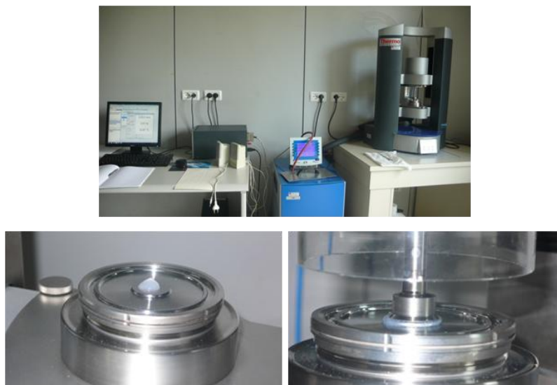
Figure 2.11: Rheometer MARS III Thermo Haake Scientific equipped with a cone-plate geometry and cone-plate angle 1°.
