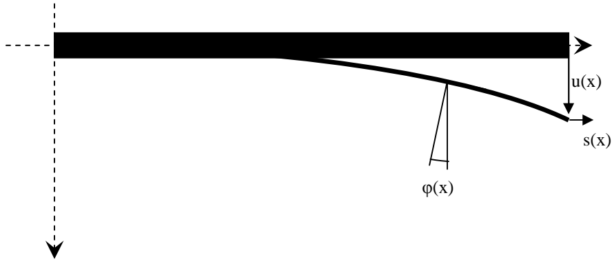
Fig. 8: Displacement in the Euler-Bernoulli Beam Theory.
