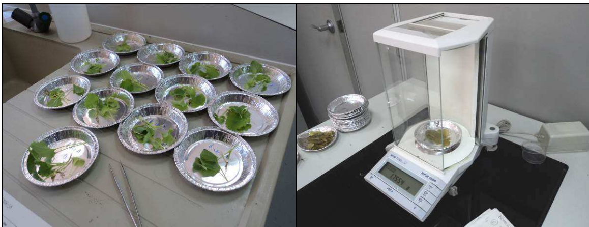
Figure 18 - Preparation of B. insularis seedlings for dry mass measure (on the left) and dry mass measure with precision balance (four decimal places) (on the right).
