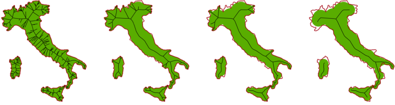
Figure 3.2: Skeletons of the map of Italy computed using SAT at growing scales (left to right). The red line denotes the boundary of the original domain. Green is the area reconstructed from the scale axis transform. Greater scales progressively ignore small features and catch only the essential parts of the shape (image courtesy of [GMPW09]).
