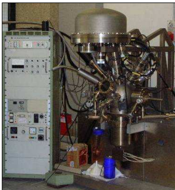
Figure 4.2 : VG ESCALAB 200, Thermo Fisher Scientific Inc., East Grinstead, UK.
