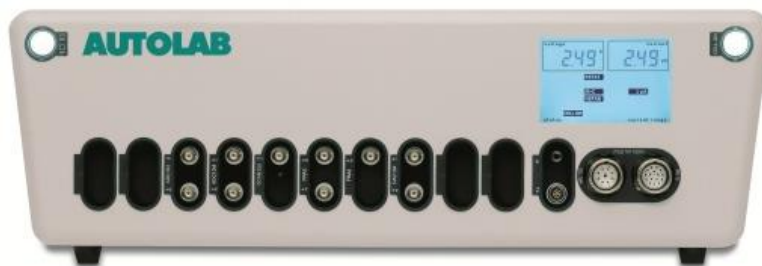
Figure 3: Metrohm Autolab 302N potentiostat-galvanostat controlled by NOVA software (Metrohm, Switzerland).
