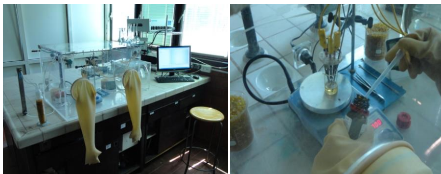
Figure 1: Nitrogen filled glove box in which all experiments were performed.
