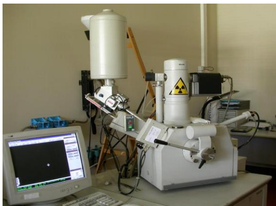
Figure 4: Scanning Electron Microscopy (SEM) equipped with Energy Dispersive X-Ray (EDX) detector (Zeiss, Germany).
