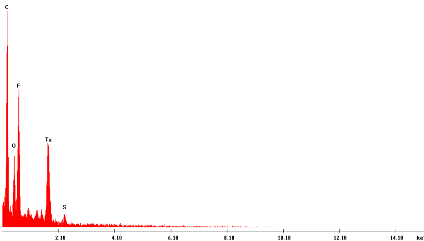
Figure 25: SEM micrograph and EDX profile of the electrodeposit formed potentiostatically on BDD in [BMP][TFSA] containing 0.25 M \text{TaF}_5 and 0.25 M LiF at potential of -1.8 V for 1 h at 125° C.
