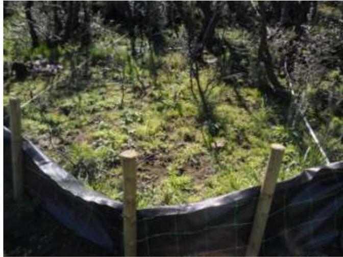
Figura 55 Silt fence sperimentale
