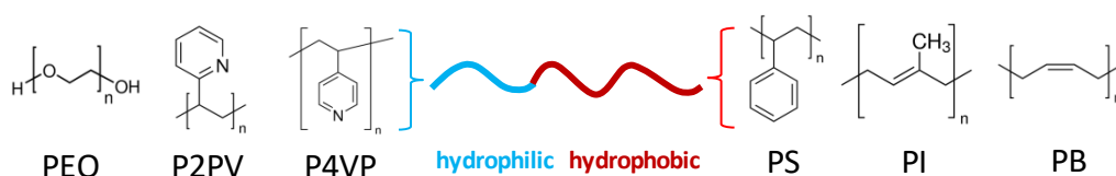
Figure 4.18 Different typologies of hydrophilic and hydrophobic block used to build block copolymers
