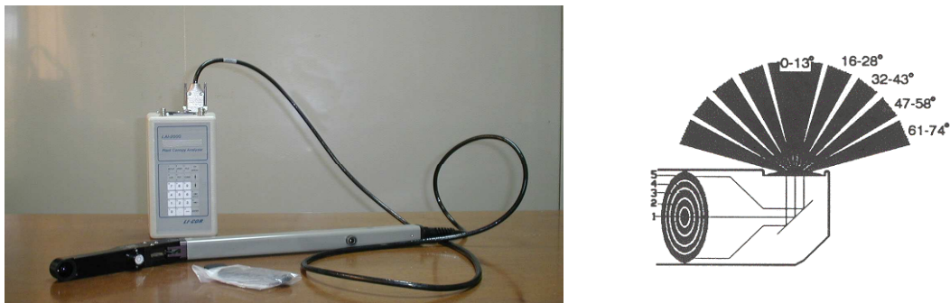
Figure 5 - LI-COR LAI 2000 Plant Canopy Analyzer and the acquisition scheme of its optical sensor.
