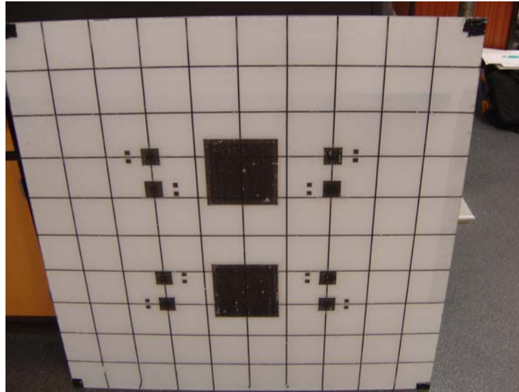
Figure 3.11 Picture of the calibration plate with the position of the magnets.
