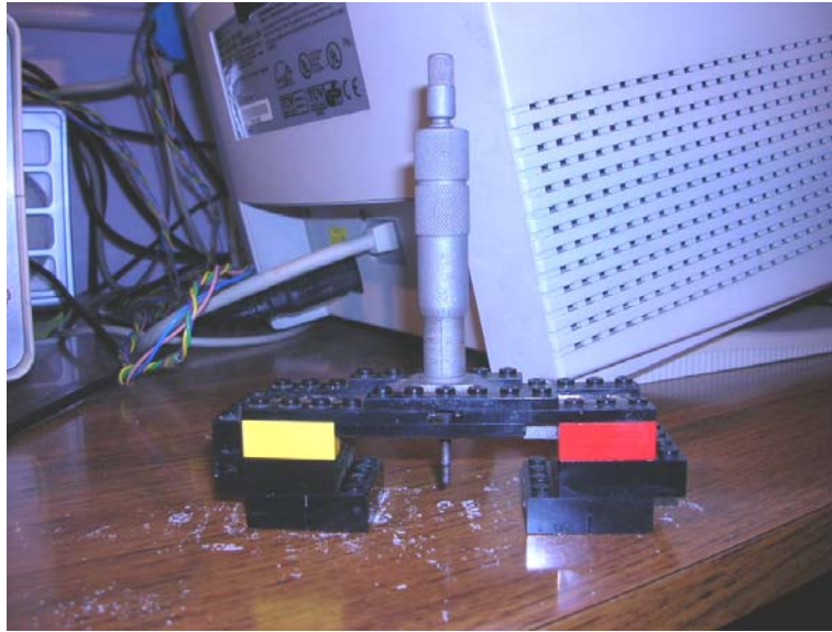
Figure 3.20 Picture of the meter tool used to check the horizontality of the brine supporting wall and the thickness of the brine layer.
