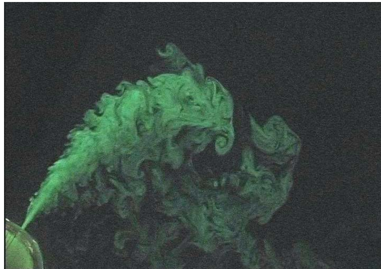
Figure 2.1 Turbulent spreading of a buoyant jet released in the sea: experiment carried out making use of Light Induced Fluorescence (LIF); as there is a linear relation between the concentration of pollutant and the light intensity, the reduction of light intensity implies the dilution of the discharged substance.
