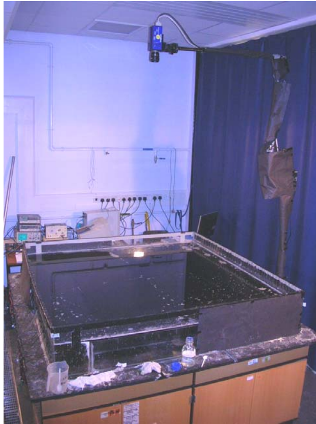
Figure. 3.3 Picture of the experimental set-up, with the tank, the camera and its stand: the black cardboard visible on the right corner of the tank and on the camera stand has the aim of reduce reflection of light coming from the lamps (visible on Figure 3.4); the working brine is made black by diluting 57 ml of black ink.
